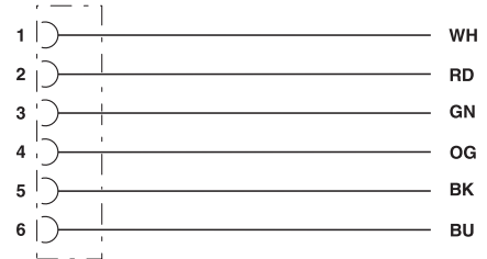
Contact assignment of 7/8" socket
