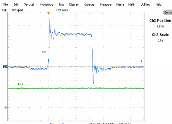
Fig. 11: Inductor node at 7A load, V_p: 0.6V , Ch 2 : LX , Ch 4 : I_{out}
