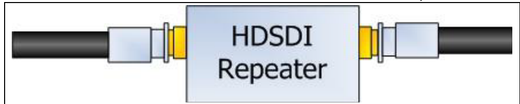
FIGURE 1-2: IN-LINE HD-SDI REPEATER (UP TO FIVE REPEATERS BEFORE ADDITIONAL POWER IS REQUIRED)
