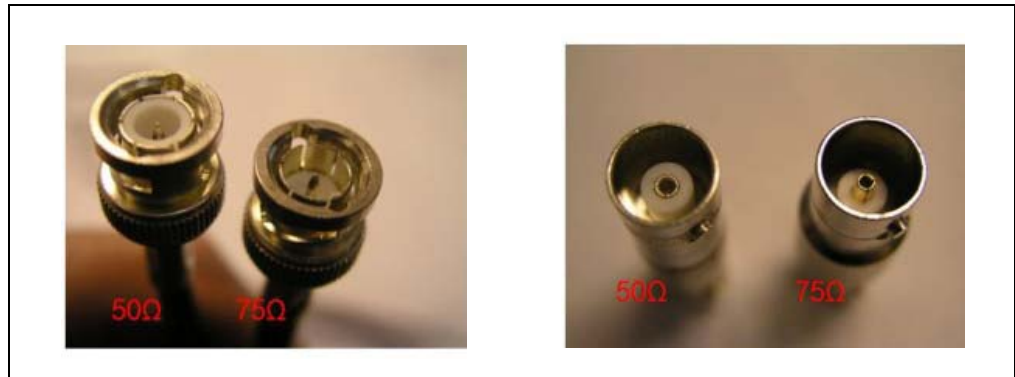
FIGURE 1-4: DIFFERENCE BETWEEN 50\Omega VS. 75\Omega CONNECTORS
