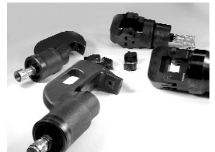
Shank-Die Line up, for wiring sizes requiring more than 14 tons [125 kN] of crimp force
