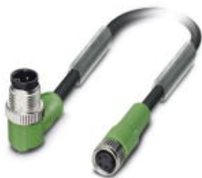
Sensor/actuator cable, 4-position, Variable cable type, Plug angled M12, A-coded, on Socket straight M8, cable length: Free input (0.2 ... 40.0 m)
