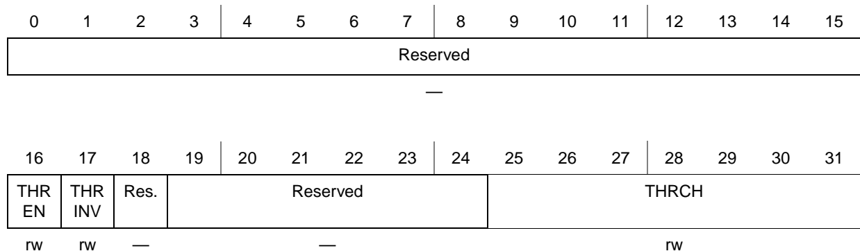
Figure 5-15. Threshold Control Register (TRCx, x = [0..3])
