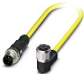
Sensor/actuator cable, 4-position, PVC, yellow, Plug straight M12 SPEEDCON, A-coded, on Socket angled M12 SPEEDCON, A-coded, cable length: 3 m
