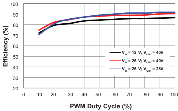
Boost Efficiency vs PWM Duty Cycle (L = 4.7μH; V DD = PWM = 5V; I OUT = 30mA/ch)
