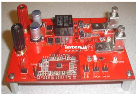
FIGURE 1. ISL8115EVAL2Z EVALUATION BOARD
