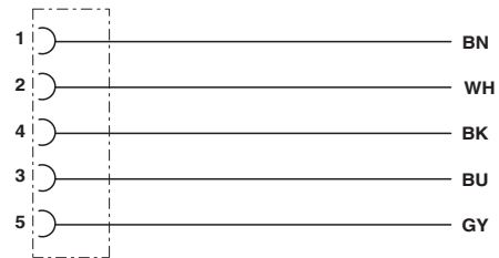
Contact assignment of the M12 socket
