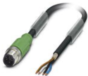
Sensor/actuator cable, 4-position, Variable cable type, shielded, Plug straight M12, A-coded, on free cable end, cable length: Free input (0.2 ... 40.0 m)
