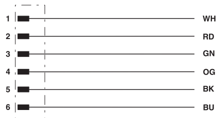
Contact assignment of 7/8" plug
