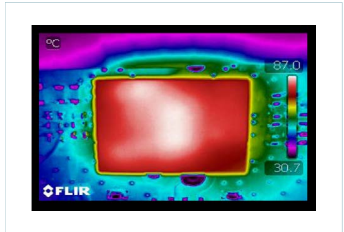
Figure 20 — Thermal Image ( V_{IN} = 24V , I_{OUT} = 4.2A , CR, OLFM Evaluation PCB)
