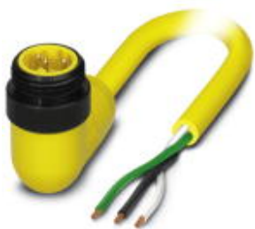
Power cable, 3-position, PVC, yellow, Plug angled 7/8"-16UNF, A - standard, on free cable end, A - standard, cable length: 2 m
