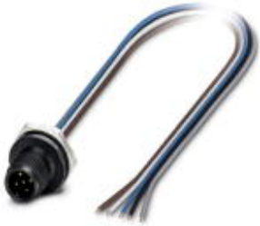
Sensor/Actuator flush-type connector, male, 5-pos., M12, A-coded, front/screw mounting with M16 thread, with 0.5 m TPE litz wire, 5 x 0.25 mm 2 , plastic version
