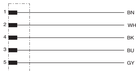
Contact assignment of the M12 plug
