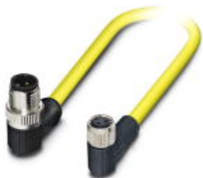
Sensor/Actuator cable, 3-position, yellow, Plug angled M12 SPEEDCON, A-coded, on Socket angled M8, Cable length: 1.5 m
