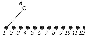
CONTACT CONFIGURATION Timing; Non-Shorting (BBM)
