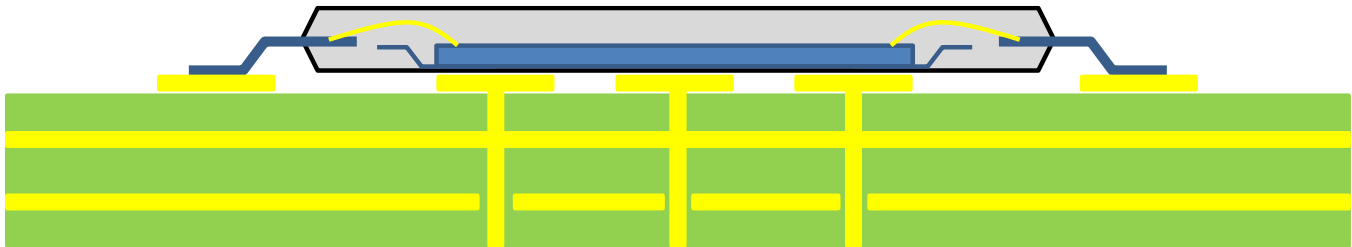
Figure10.2-1: Example thermal via holes on PCB.
