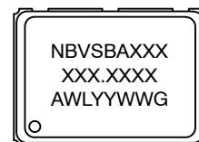
6 PIN CLCC LN SUFFIX CASE 848AB
