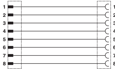
Contact assignment of M12 connector/socket
